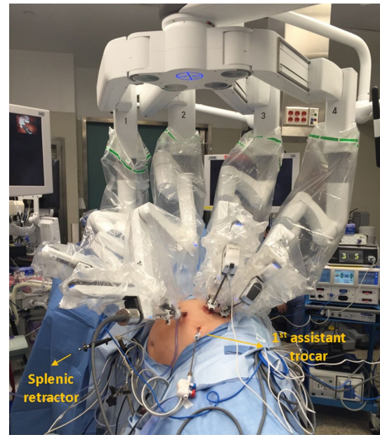
Fig. 2 Intraoperative photo demonstrating the 4-arm robotic transabdominal lateral left adrenalectomy technique in an obese patient. In addition to four robotic arms, a splenic retractor and a 1st assistant trocar are introduced. Robotic arms 1 and 4 operate the graspers, arm 2 holds the camera, and arm 3 operates the vessel sealer
